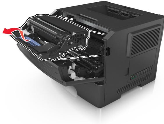
**Warning—Potential Damage:** Do not touch the shiny blue photoconductor drum under the imaging unit. Doing so may affect the quality of future print jobs.
