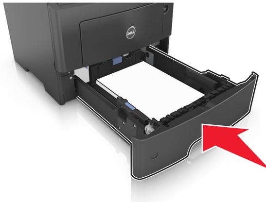
**7** From the printer control panel, set the paper size and type in the Paper menu to match the paper loaded in the tray.
