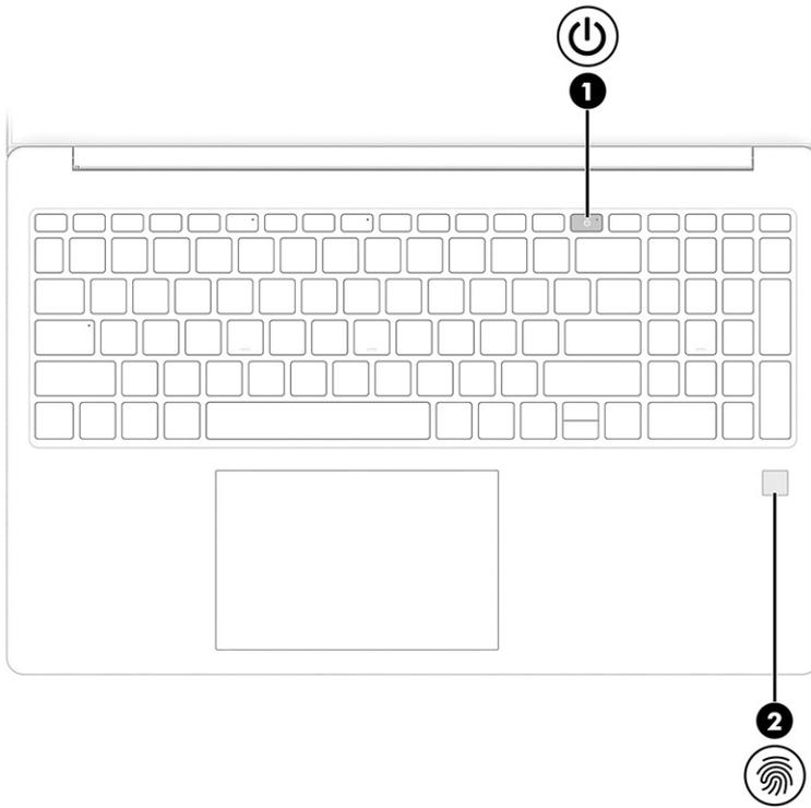
Fingerprint readers, which enable a fingerprint logon, can be located on the touchpad, on a side panel of the computer, or on the top cover below the keyboard.
