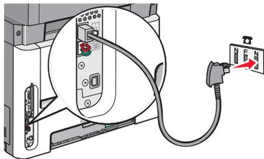
**4** If you would like to use the same line for both fax and telephone communication, then connect a second telephone line (not provided) between the telephone and the F slot of an active analog telephone wall jack.
