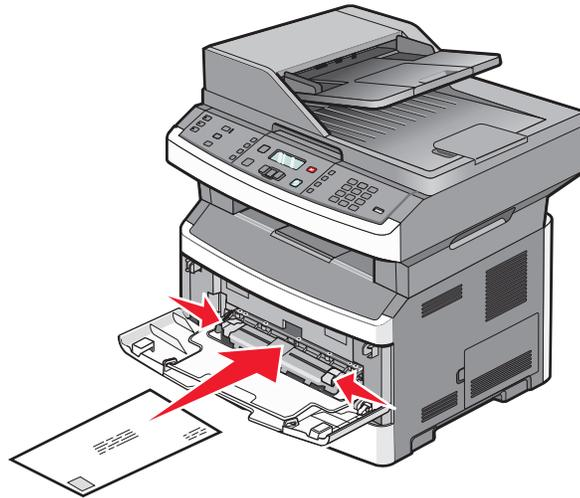
**3** Feed paper into the manual feeder only to the point where its leading edge can contact the paper guides.
