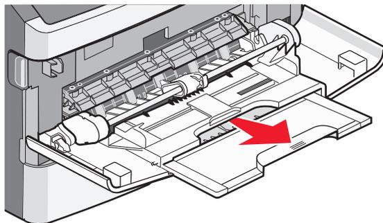
3 Pull the extension so it flips forward and down.
