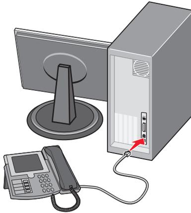
5 Connect an additional telephone cord (not provided) from the computer modem to the printer EXT port
