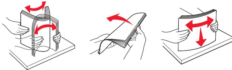
**4** Load the paper stack toward the back of the tray as shown with the recommended print side facedown.
