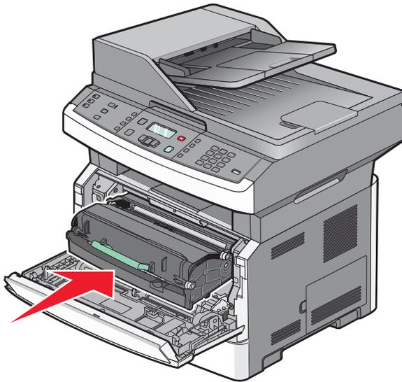
**8** After you replace the photoconductor kit, reset the photoconductor counter. To reset the counter, see the instruction sheet that came with the new photoconductor kit.
