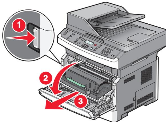
**4** Lift the flap at the front of the printer, and then remove any jammed sheets.
