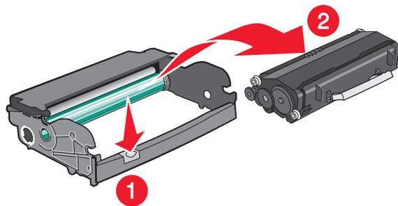
5 Unpack the new photoconductor kit. Be careful not to touch the photoconductor drum.
