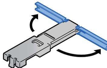
**4 Attach the envelope feed guide as shown in the illustration.**
