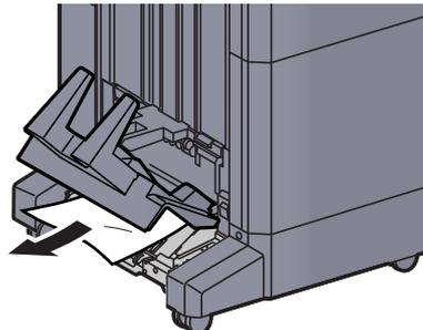
**3 Press the release lever to pull the folding unit out.**
