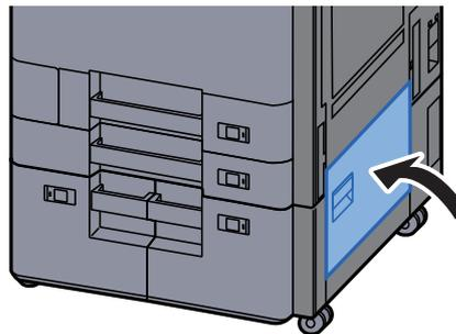
**5 If the optional side feeder is installed, return the side feeder to the original position.**
