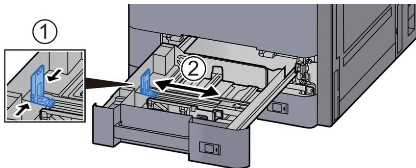
**6 Adjust the position of the paper width guides located on the left and right sides of the cassette.**
