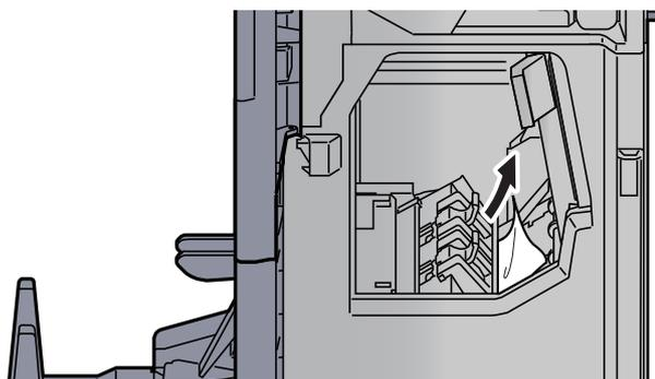
**3 Remove the Staple Cartridge Holder (B) or (C).**
