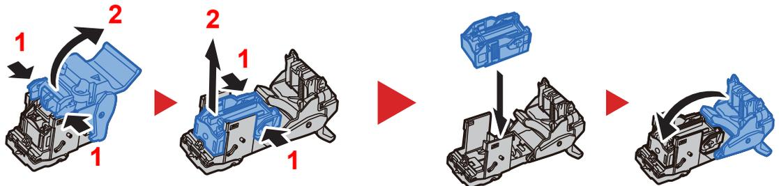
**4 Install the Staple Cartridge Holder (B) or (C).**
