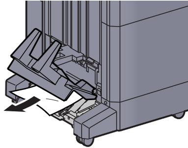
**9 Press the release lever to pull the folding unit out.**
