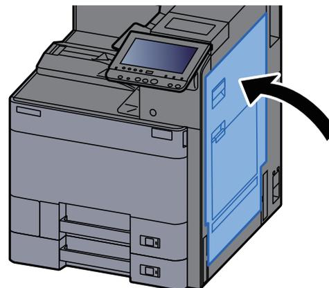
**17** If the optional side feeder is installed, return the side feeder to the original position.
