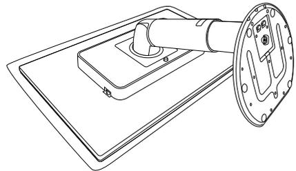
3. While keeping the release button pressed, tilt the base and slide it out.
