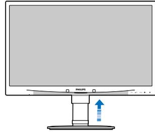
2. Place the monitor face down on a smooth surface, taking care to avoid scratching or damaging the screen. Then lift the monitor stand.
