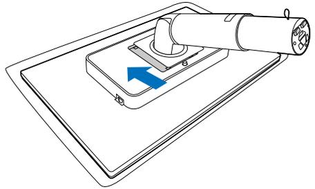
3. Hold the monitor base stand with both hands and firmly insert the base stand into the base column.
