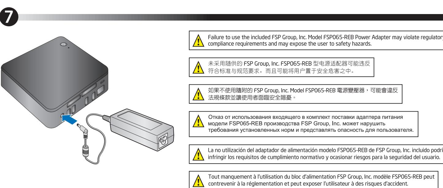
**Failure to use the included FSP Group, Inc. Model FSP065-REB Power Adapter may violate regulatory compliance requirements and may expose the user to safety hazards.**
