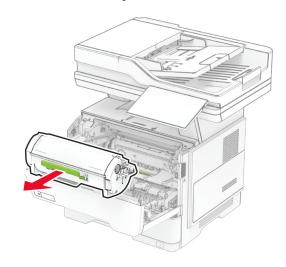
Remove the used imaging unit.
