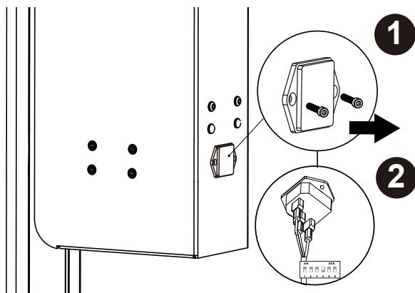
3. Open the battery cover of the handset, there is a 6-Digit DIP SWITCH inside.
