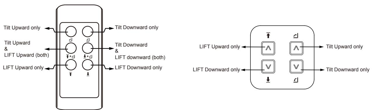
Designated Remote control shall be compatible with specific motorized cart
