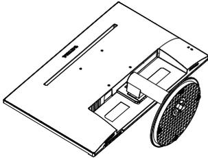
2. Press the release button to detach the base stand away from the base column.
