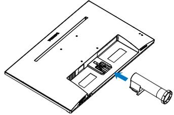
2. Hold the monitor base stand with both hands and firmly insert the base stand into the base column.
