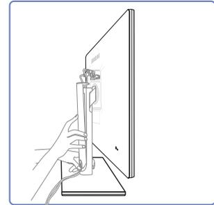
Hold the cover stand rear with right hand, and fix the cable into the groove in the cover stand rear with left hand.
