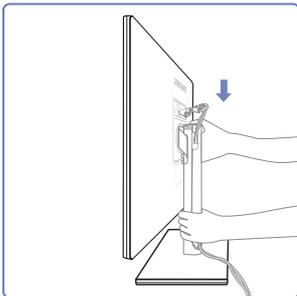
Hold the bottom of the stand bar securely with left hand, steadily hold the top of the stand bar with right hand, then use the thumb of right hand to press and push the cover stand rear downward.
