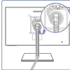
Install the cables into the holder cable at the right side.
