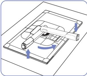
Place a protective cloth or cushion on a flat surface. Next, place the product with the face down on top of the cloth or cushion. rotate the stand body about 90°
