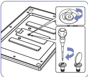
Tightly fasten the screw to the bottom of the base.
