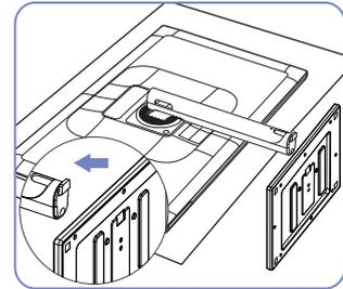
Insert the stand base into the stand body in the direction of the arrow.
