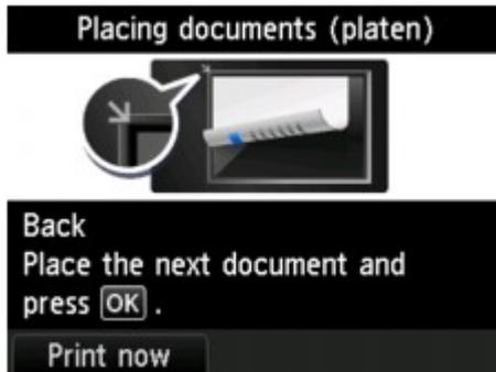
Remove the sheet of original from the platen glass after scanning and load the next sheet on the platen glass, then press the **OK** button.
