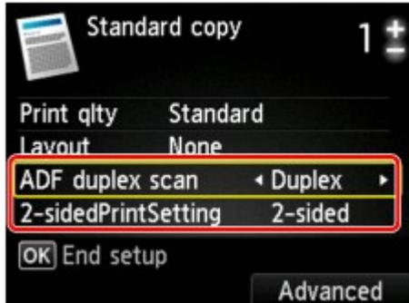
Specify the place to load originals or copy settings according to the two-sided copying method.
