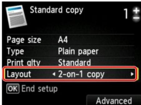
Press the right **Function** button to specify the orientation and the advanced layout.
