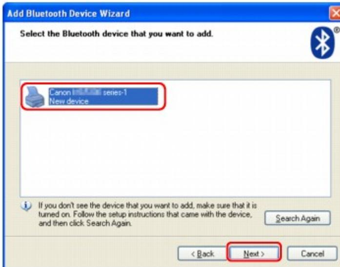
Select the same device name as that checked under [Checking the Device Name of the Printer](#).
