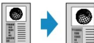
If you select other than **Fit to page** and press the right **Function** button, **Magnification** screen is displayed. Use the ▲▼ button to specify the magnification.
