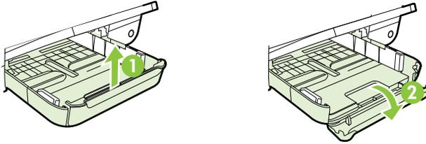
4. Insert the media print-side down along the right of the main tray. Make sure the stack of media aligns with the right and back edges of the tray, and does not exceed the line marking in the tray.
