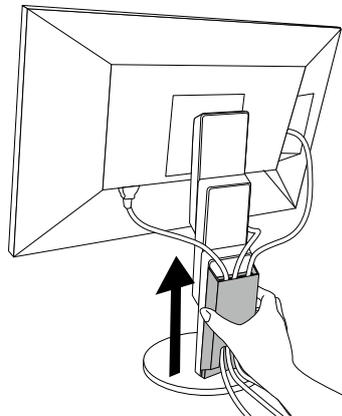
2. While holding down
