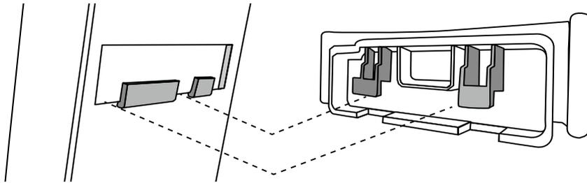
2. Slide the cable holder to the right, and attach it to the stand.
