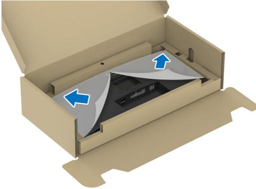
**7.** Attach the stand assembly to the display.
