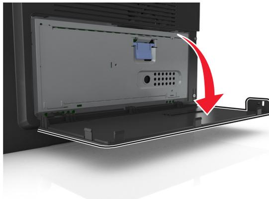
2 Lightly press the stop on the left side of the access door, and then slide the access door to remove it.
