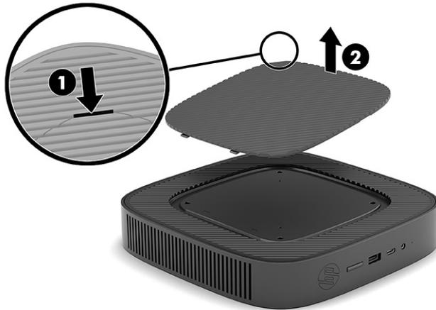
3. Set the thin spacer into the depression on the right side of the thin client.
