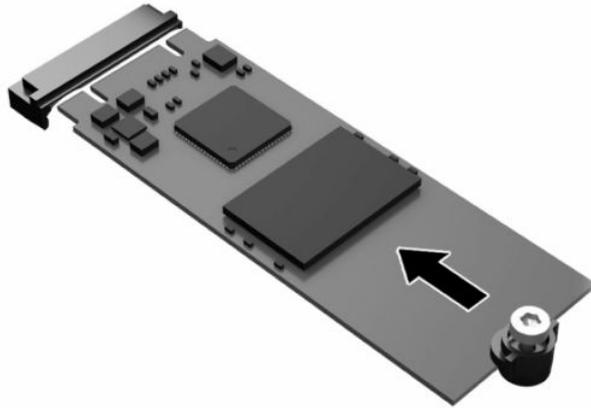
7. Press the storage module down and use a screwdriver to tighten the screw and secure the module to the system board.
