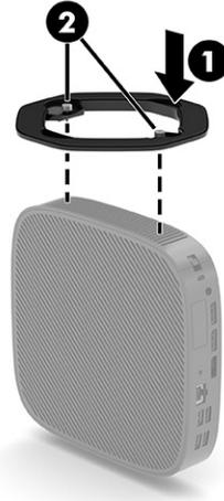
5. Horizontal orientation: Attach the stand to the right side of the thin client.
