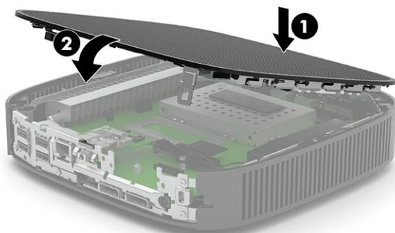
2. Insert the hooks on the left side of the rear I/O panel (1) into the left side of the back of the chassis, rotate the right side (2) to the chassis, and then press the right side into the chassis until it locks in place.
