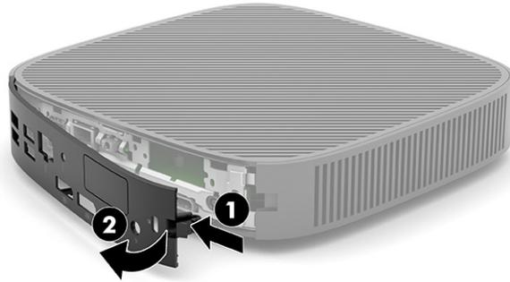
7. Press the latch (1) that secures the access panel to the chassis.
