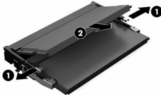
4. Slide the new memory module (1) into the socket at approximately a 30° angle, and then press the memory module down (2) so that the latches lock it in place.
