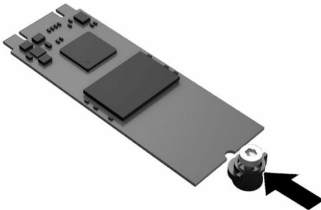
6. Slide the new storage module into the M.2 socket on the system board and press the module connectors firmly into the socket.
