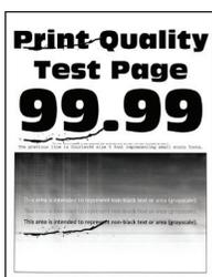
**Note:** Before solving the problem, print the Print Quality Test Pages. From the control panel, navigate to **Settings > Troubleshooting > Print Quality Test Pages**. For non-touch-screen printer models, press
