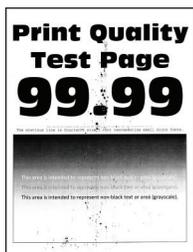
**Note:** Before solving the problem, print the Print Quality Test Pages. From the control panel, navigate to **Settings > Troubleshooting > Print Quality Test Pages**. For non-touch-screen printer models, press
