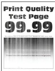
**Note:** Before solving the problem, print the Print Quality Test Pages. From the control panel, navigate to **Settings > Troubleshooting > Print Quality Test Pages**. For non-touch-screen printer models, press
