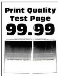
**Note:** Before solving the problem, print the Print Quality Test Pages. From the control panel, navigate to **Settings > Troubleshooting > Print Quality Test Pages**. For non-touch-screen printer models, press
