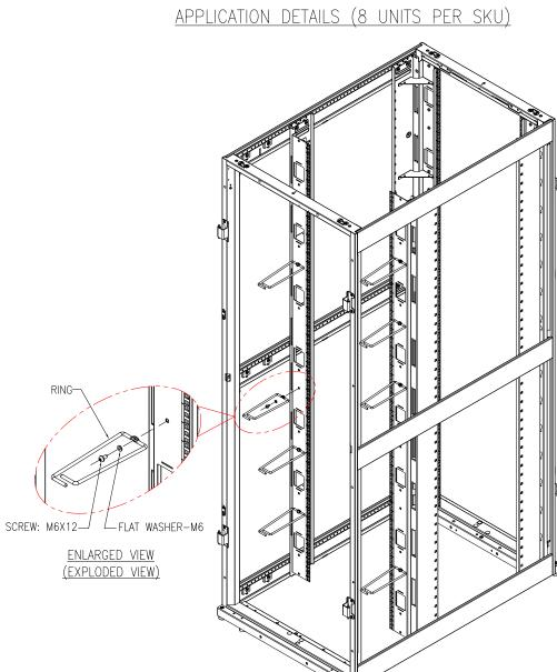
TYPICAL APPLICATION, DOORS & SIDE PANELS NOT SHOWN (ISOMETRIC VIEW)
