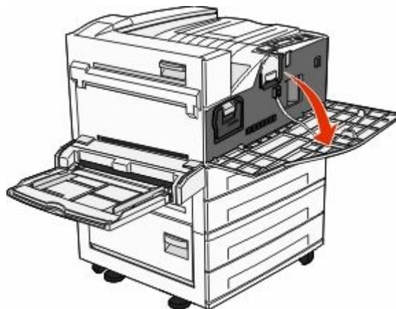
3 Grasp the handle and pull out the cartridge.
