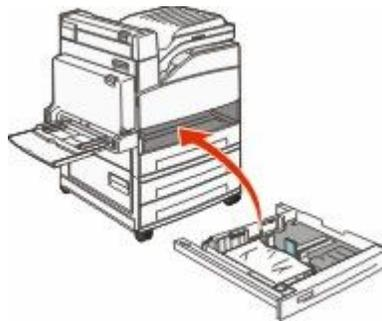
**7** If the paper type you loaded differs from the type that was previously loaded in the tray, then change the Paper Type setting for the tray.
