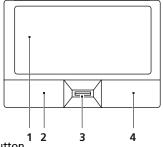
Use Acer Bio-Protection fingerprint reader (3) supporting Acer FingerNav 4-way control function (only for certain models) to scroll up or down and move left or right a page. This fingerprint reader or button mimics your cursor pressing on the right scroll bar of Windows applications.
