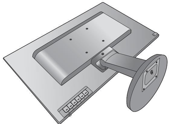
Release the screw that fixes the stand to the monitor. Use of a flat-head screwdriver is recommended. Then pull the monitor stand backward away from the monitor.
