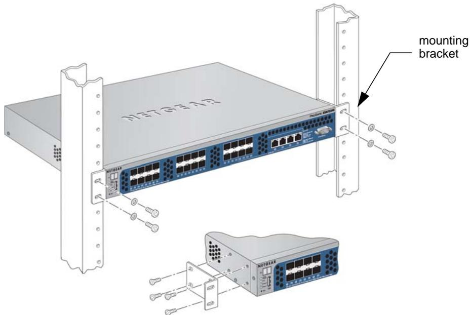
**Figure 1. Installing the Switch in a Rack**
