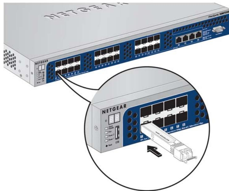
**Figure 3. Insert the SFP+ or SPF Module into the Switch**
