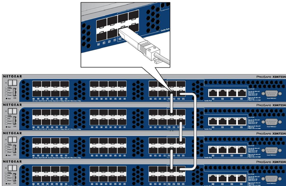
Figure 4. Switch Stack
