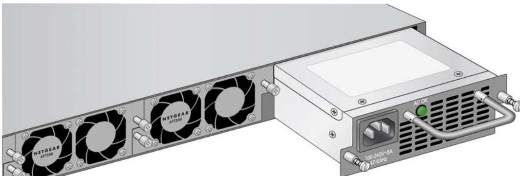
**Figure 5. Insert the Power Supply Module**
