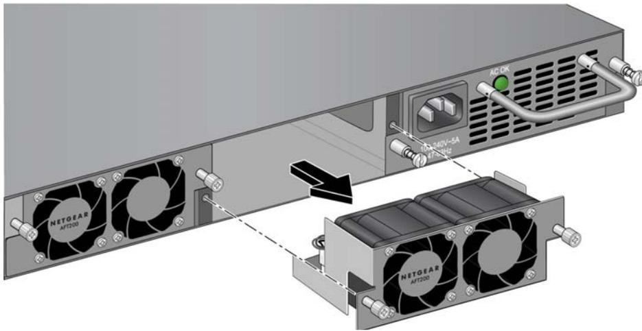
Figure 6. Fan Tray Removal
