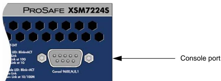
**Figure 7. Rear Panel Console Port**
