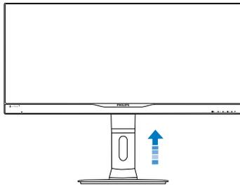
2. Place the monitor face down on a smooth surface. Pay attention not to scratch or damage the screen. Then lift the monitor stand.
