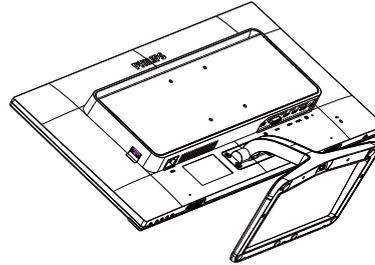
2. Use your fingers to loosen the screw located at the bottom of the base, and then remove the base from the stand.
