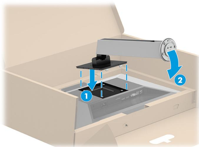
3. With the monitor still placed facedown inside the box, insert the base into the bottom of the monitor stand (1), and then swivel the base counterclockwise to lock it in place (2). Confirm that the arrow on
