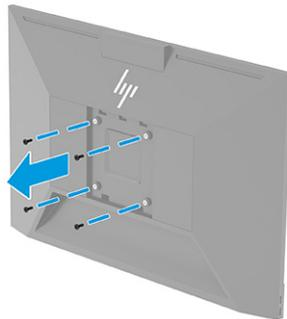
2. To attach the monitor head to a swing arm or other mounting device, insert four mounting screws through the holes on the mounting device and into the VESA screw holes on the back of the monitor head.
