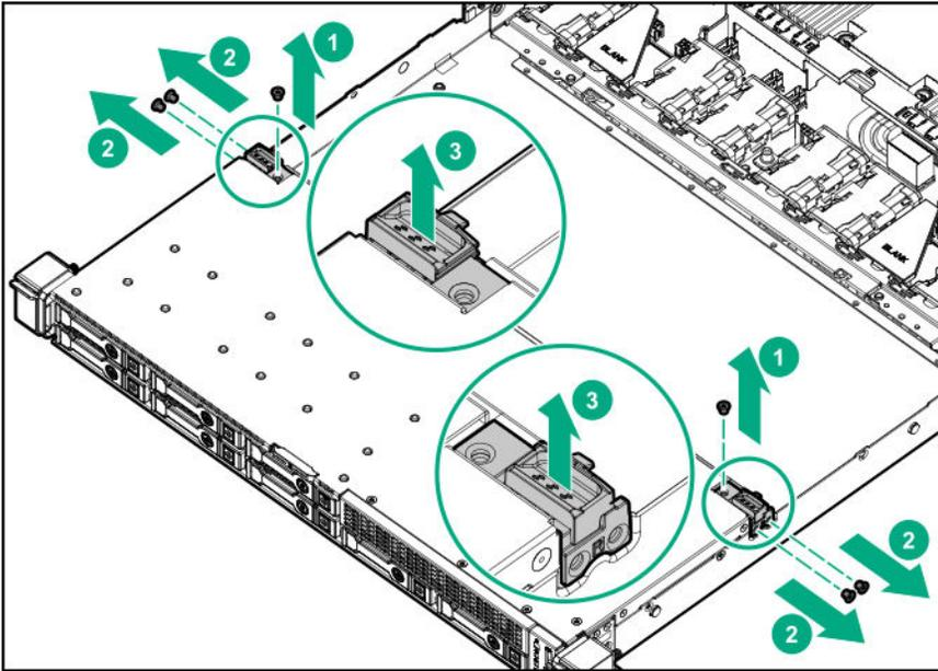
**14.** Remove the outer drive cage.
