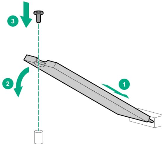
10. **Install the M.2 SSD enablement board.**
