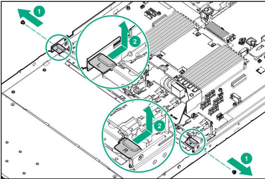
10. Remove all the existing single rotor fans and fan blanks.
