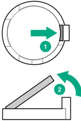
9. Insert the battery with the "+" side facing up on the socket, and then press the battery down to secure it in place.
