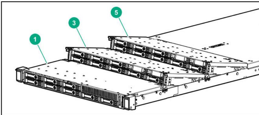
**NOTE:** 2SFF drive cage is not supported in long chassis configuration.
