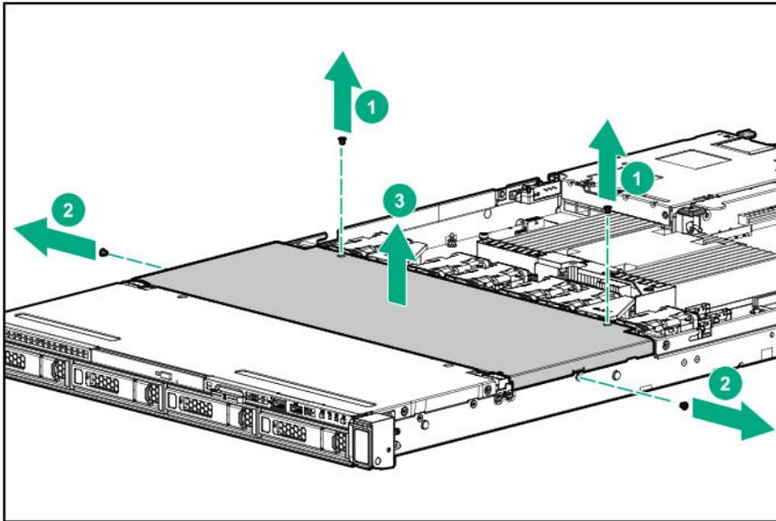
9. Remove the outer drive cage cover.
