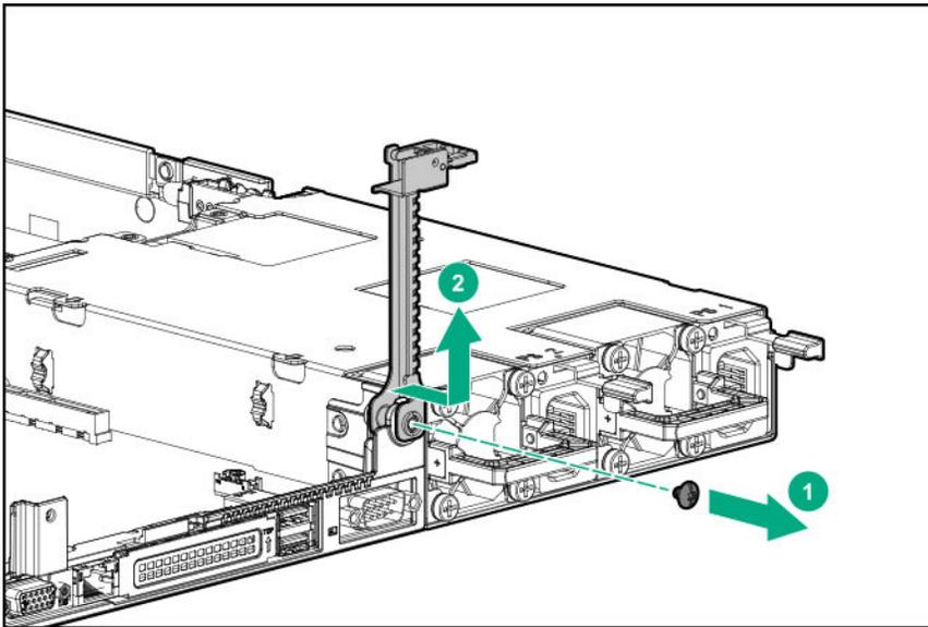
12. Install the full-height PCIe bracket.
