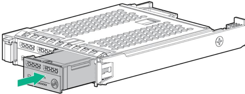
2. To install a drive in outer drive cage, **remove the bezel** if installed.
