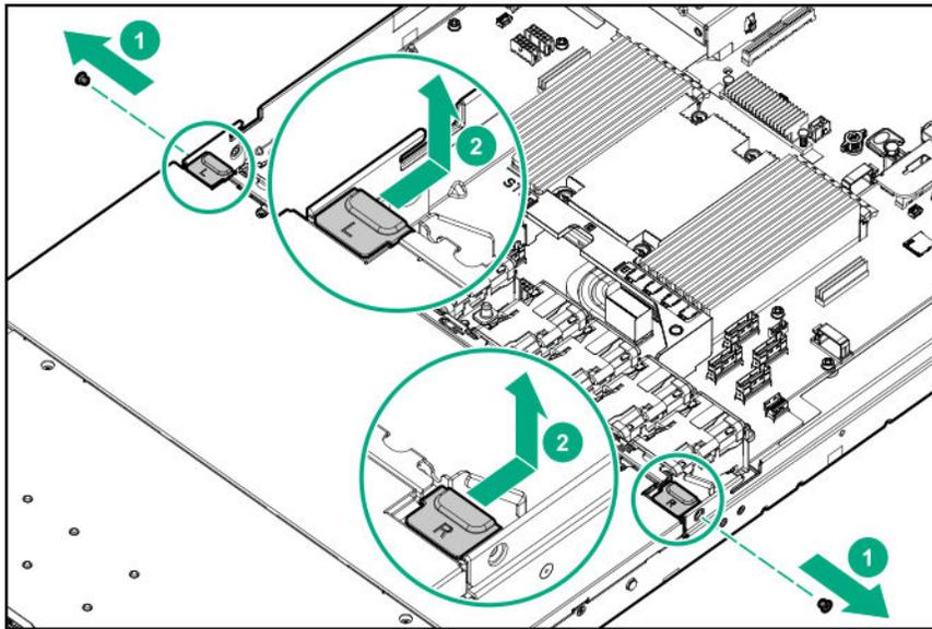
**10.** Remove the inner drive cage.
