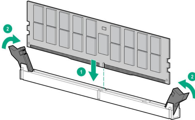
The DIMM slots are structured to ensure proper installation. If you try to insert a DIMM but it does not fit easily into the slot, you might have positioned it incorrectly. Reverse the orientation of the DIMM and insert it again.
