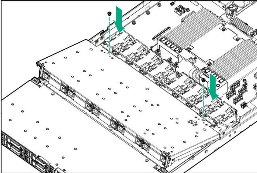
2. If removed, **install the drives in the inner drive cage.**
