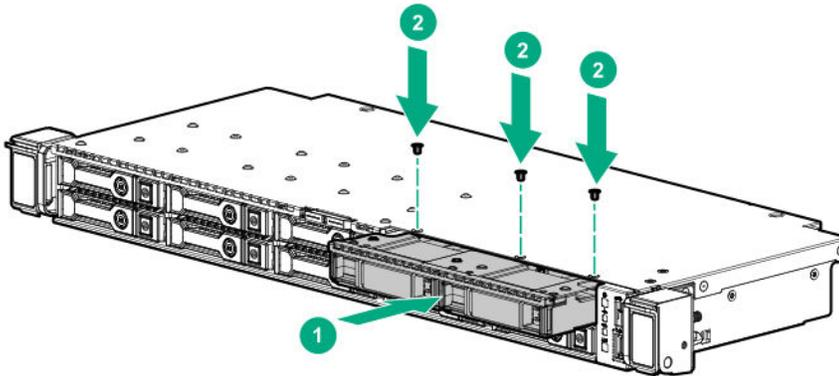
11. Remove the cable guard:
