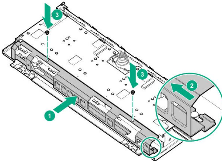
**14.** **Install the outer drive cage.**
