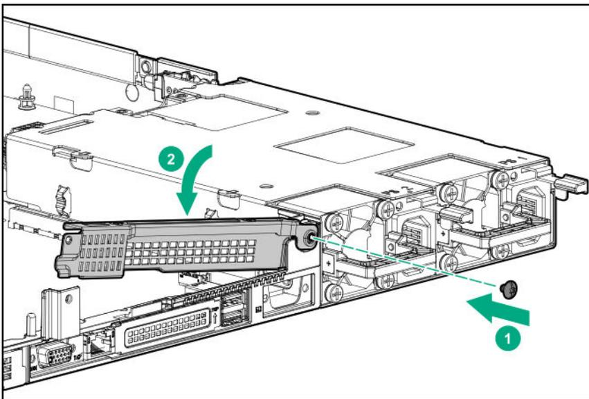
13. Install the secondary riser cage:
