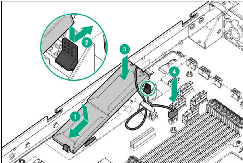
9. **Connect the controller backup power cable.**
