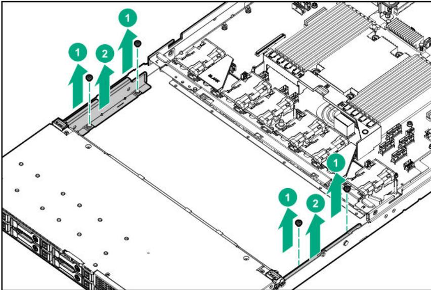
**13.** Remove the drive cage latches.
