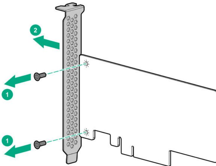
8. Install the low-profile bracket on the controller.
