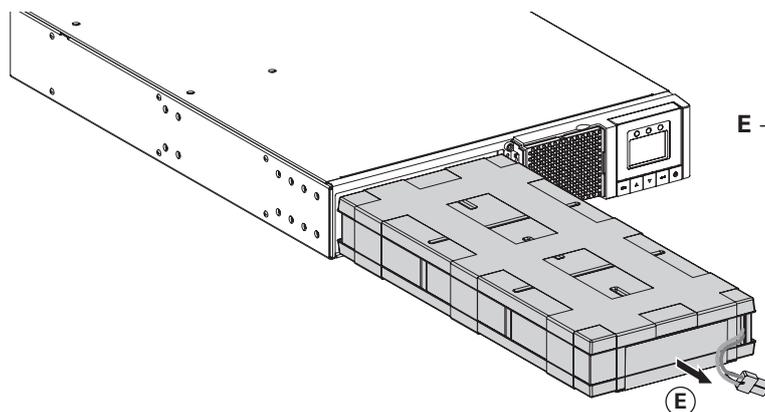
**E** - Pull the plastic tab to remove the battery block and replace it.
