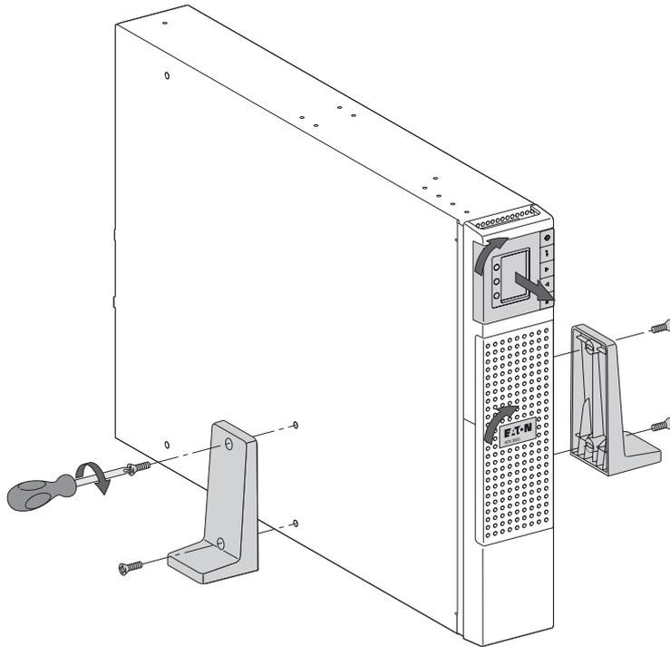
**Note.** The two supports for the tower position are used on the RT 2U version only.
