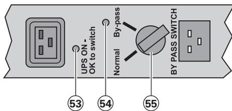
The HotSwap MBP module has a rotary switch (55) with two positions:
