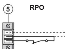
Contact open: UPS shutdown, LED  $\triangle$  goes ON.
