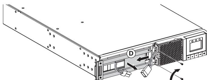
**D** - Remove the metal protection cover in front of the battery (two screws).
