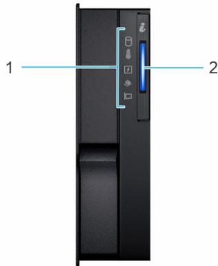
Figure 7. Left control panel
