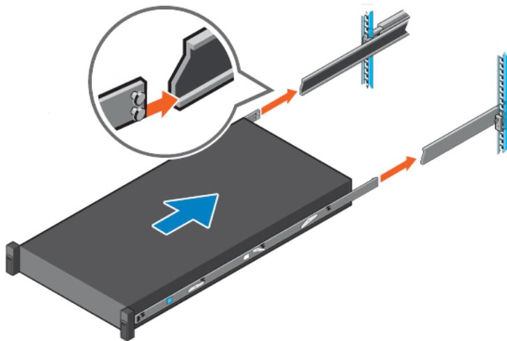
**Figure 33. Install system into the extended rails**
