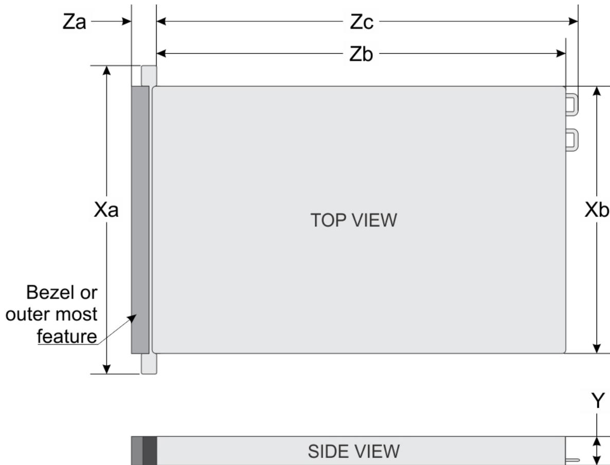
Figure 35. Chassis dimensions
