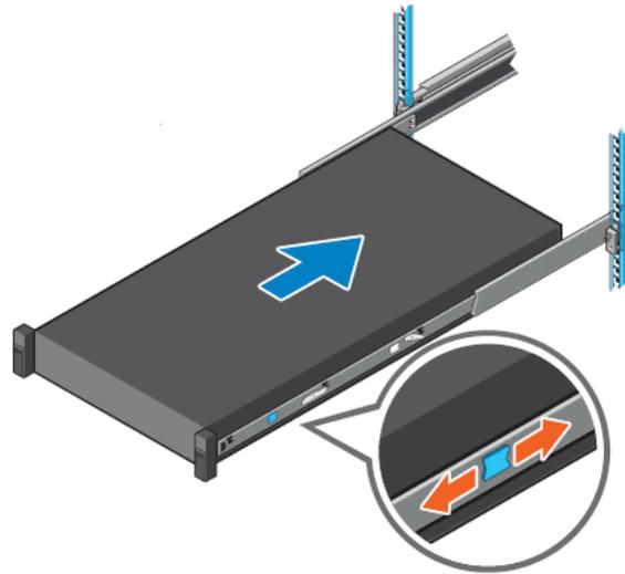
**Figure 30. Slide system into the rack**
