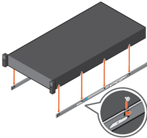
**Figure 32. Attach the inner rails to the system**
