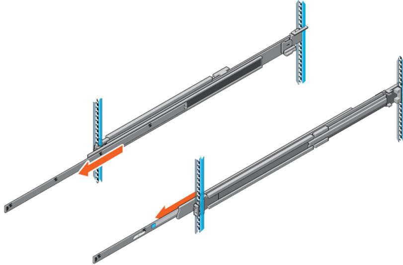
**Figure 28. Pull out inner rail**
