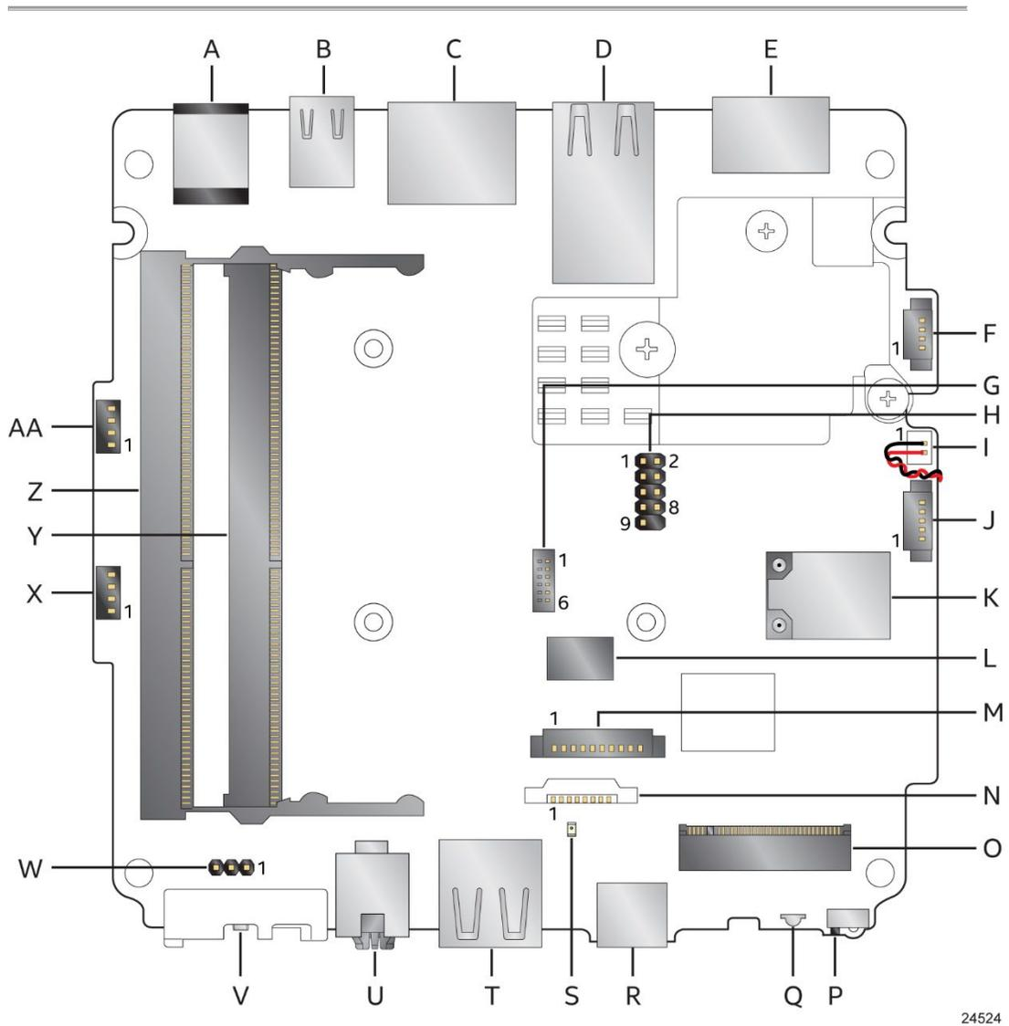
Figure 1. Major Board Components (Bottom) with Pin 1 Indicators
