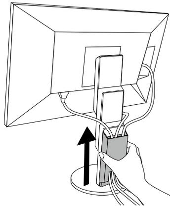
2. While holding down
