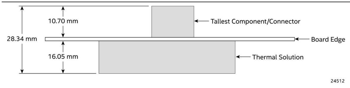
Figure 21. Board Height Dimensions
