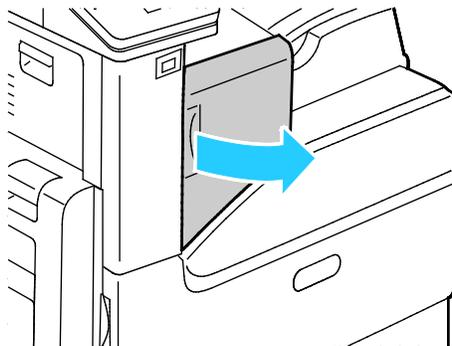
2. To remove the staple cartridge, grasp the orange handle, then pull it firmly toward you.
