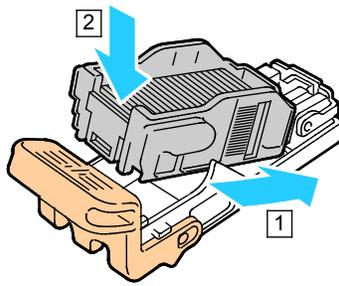
7. Grasp the staple cartridge by the orange handle, then insert the cartridge into the stapler until it clicks.
