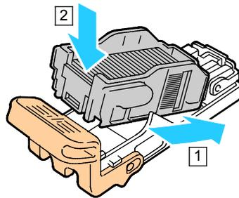
6. Grasp the new staple cartridge by the orange handle, then insert the cartridge into the stapler until it clicks.
