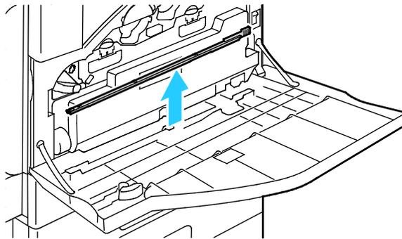
4. Slowly push the cleaning rod into the printer until it stops, then pull it out. Repeat this action two more times.
