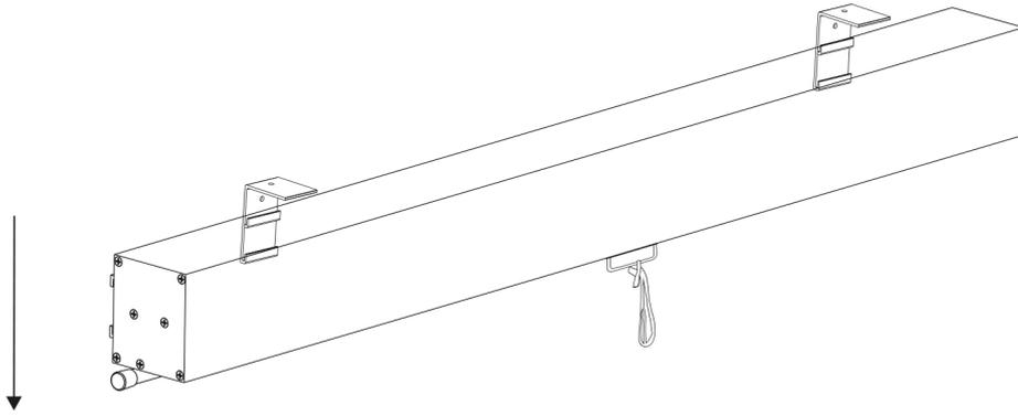
Mount the projection screen on the two hooks
