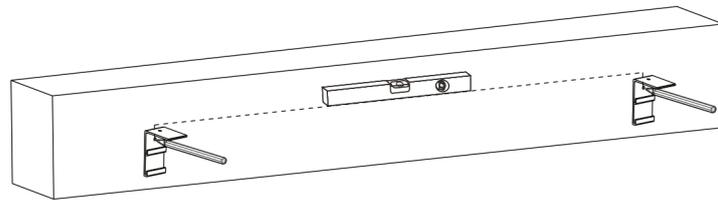
Make sure that the hooks are in level by bubble level
