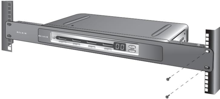
**Note:** If this PRO3 KVM Switch will be daisy-chained to another KVM switch, set the BANK address prior to installing on a rack. Refer to the section titled “Connecting Multiple PRO3 KVM Switches (Daisy-Chaining)” in this User Manual.
