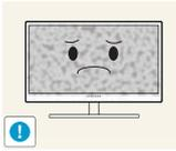
Leaving the screen fixed on a stationary image for an extended period of time may cause afterimage burn-in or defective pixels.
