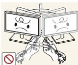
Do not lift or move the product by pulling the power cord or any cable.
