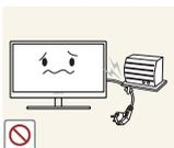
Do not bend or pull the power cord with force. Do not weigh the power cord down with a heavy object.
