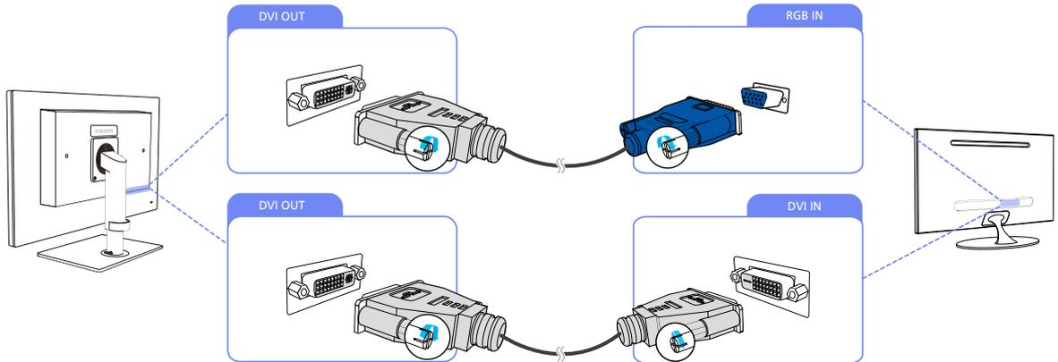
1 Connect [DVI OUT] on the product to [DVI IN] or [RGB IN] on another monitor using a DVI or DVI to D-SUB cable.
