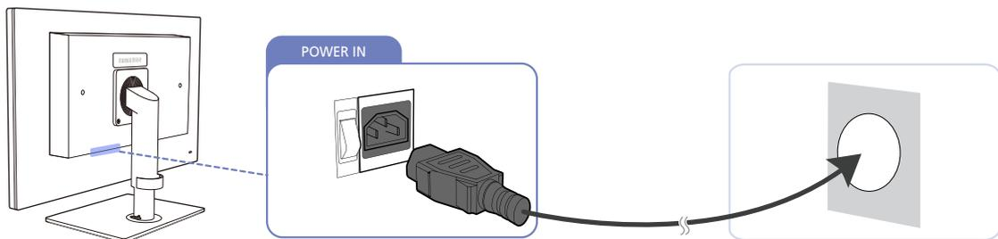
1 Connect the power cable to the product and the power outlet, then turn on the power switch. (The input voltage is switched automatically).
