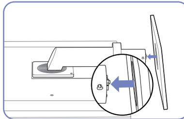
Insert the stand base into the stand in the direction of the arrow.
