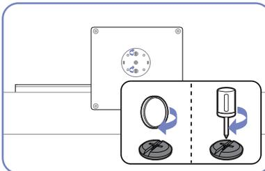
Fasten the screw tightly (using a screwdriver or coin) into the bottom of the base.
