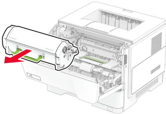
3 Remove the used imaging unit.
