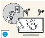
If the product generates a strange noise, a burning smell, or smoke, remove the power cord immediately and contact Samsung Customer Service Center (page 88).
