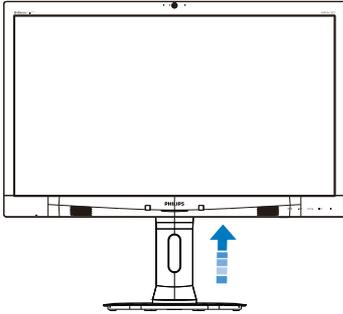
2. Place the monitor face down on a smooth surface. Pay attention not to scratch or damage the screen. Then lift the monitor stand.
