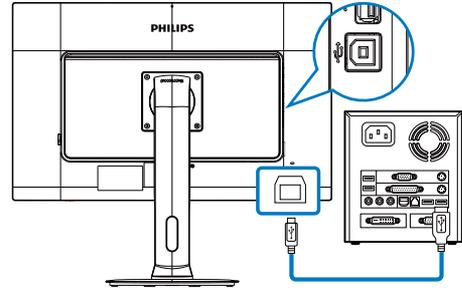
1. Connect your USB cable to upstream of USB hub on the side IO of monitor from PC side.
