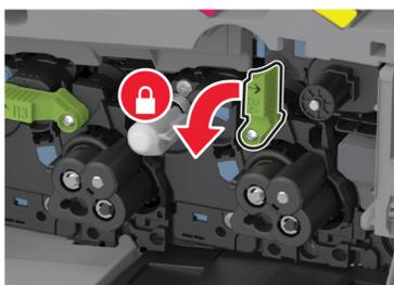
**8** Remove the printhead wiper, and then clean the printhead lenses.
