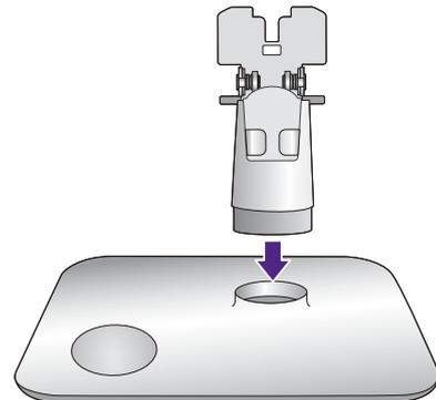
Tighten the thumbscrew on the bottom of the monitor base as illustrated.
