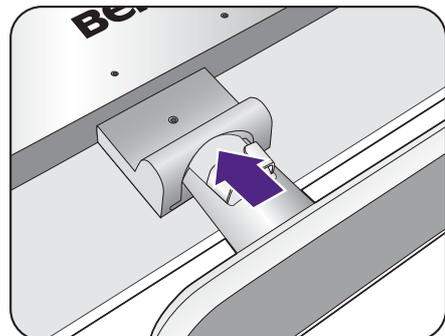
Carefully lift the monitor, turn it over and place it upright on its stand on a flat even surface.
