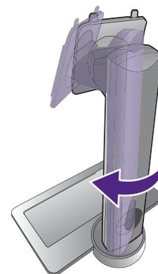
Tighten the thumbscrew on the bottom of the monitor base as illustrated.
