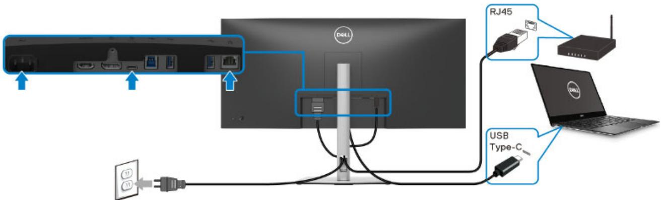
**Connecting/ disconnecting the SuperSpeed USB 5 Gbps (USB 3.2 Gen1) cable and Power cable**
