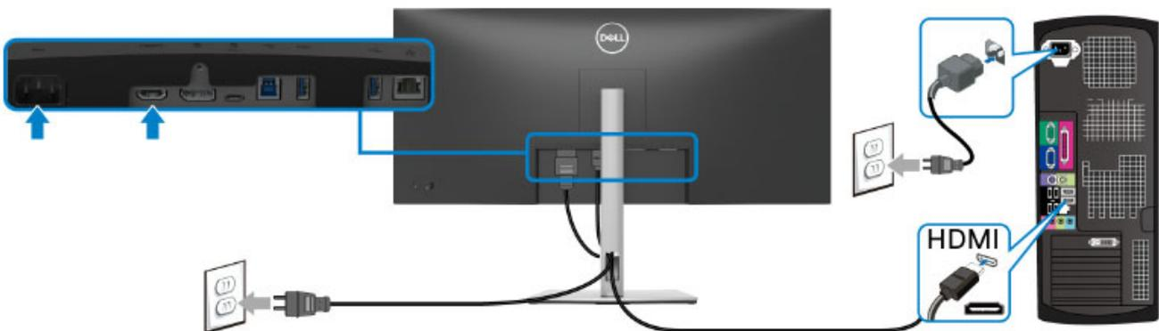
**Connecting/ disconnecting the USB Type-C cable and Power cable**
