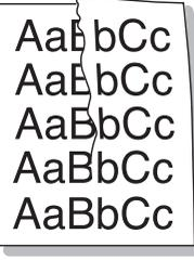
A diagram showing five lines of text: 'A a B b C c'. The lines are distorted and appear to have vertical creases or wrinkles, illustrating the condition of page wrinkles or creases. | <ul style="list-style-type: none"><li>• Ensure that the paper is loaded properly.</li><li>• Check the paper type and quality.</li><li>• Turn the stack of paper over in the tray. Also try rotating the paper 180° in the tray.</li></ul>                                                          |
