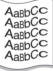
A diagram showing five lines of text: 'A a B b C c'. The lines are curved upwards at both ends, illustrating the condition of page curl or wave.                                               | <ul style="list-style-type: none"><li>• Ensure that the paper is loaded properly.</li><li>• Check the paper type and quality. Both high temperature and humidity can cause paper curl.</li><li>• Turn the stack of paper over in the tray. Also try rotating the paper 180° in the tray.</li></ul> |
