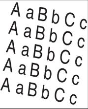
A diagram showing five lines of text: 'A a B b C c'. Each line is progressively more tilted to the right than the one above it, illustrating the condition of page skew.                          | <ul style="list-style-type: none"><li>• Ensure that the paper is loaded properly.</li><li>• Check the paper type and quality.</li><li>• Ensure that the guides are not too tight or too loose against the paper stack.</li></ul>                                                                   |
