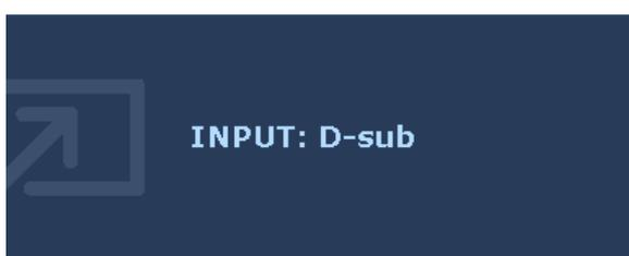
Press the **ENTER** key to toggle between different PC video signal inputs that may be connected to your monitor.
