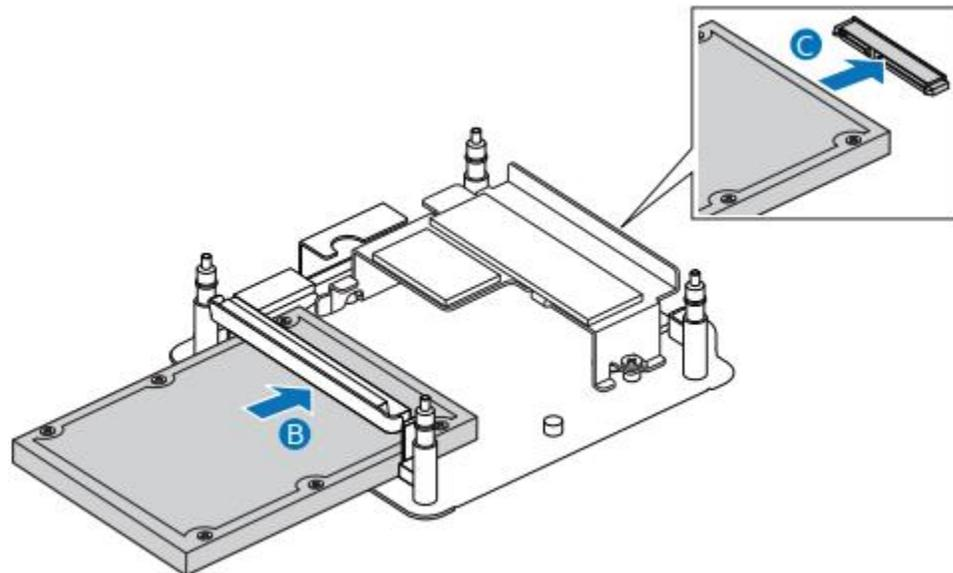
2. Secure the drive into the drive bay with the two small silver screws that were included in the box. Set the drive bay bracket down inside the chassis.
