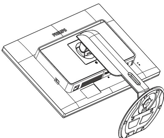
2. While keeping the release button pressed, tilt the base and slide it out.
