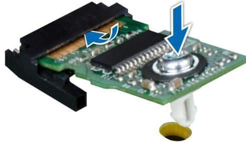
Figure 108. Installing the TPM
