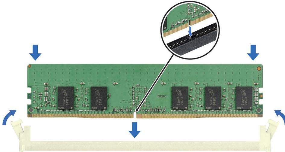
**Figure 54. Installing a memory module**
