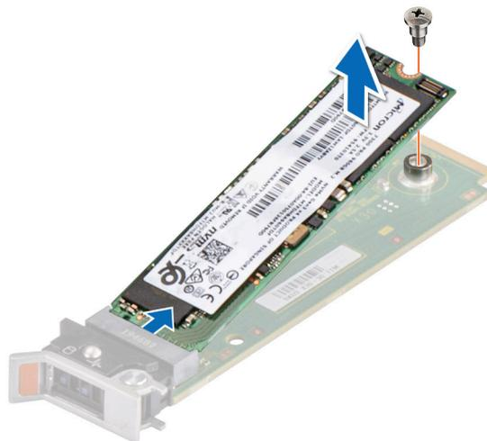
**Figure 75. Removing the M.2 SSD**
