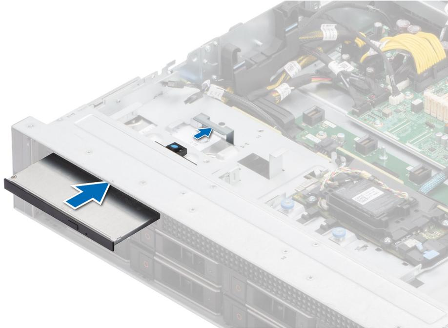
**Figure 114. Installing the ODD**
