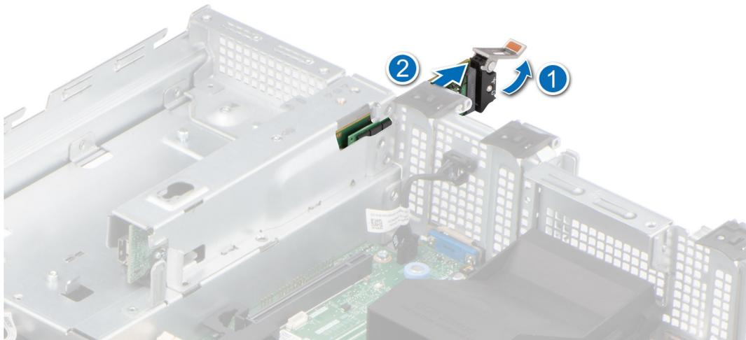
**Figure 74. Removing the BOSS S2 card carrier**
