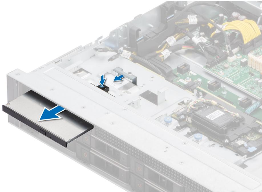
Figure 113. Removing the ODD
