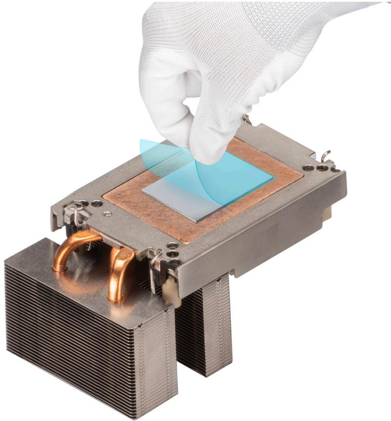
**Figure 63. Remove the Thermal Interface Material (TIM) protective film**
