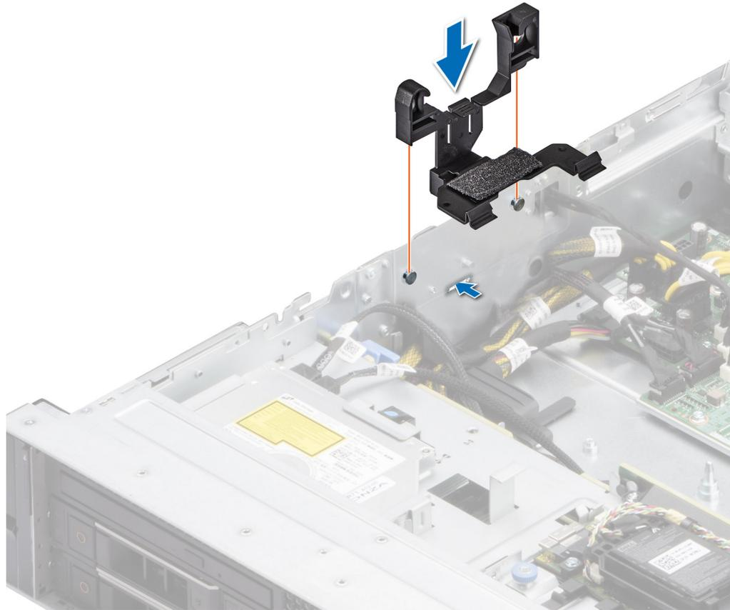
**Figure 31. Installing the side wall bracket**
