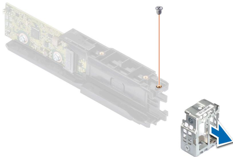
**Figure 79. Removing the BOSS cover**
