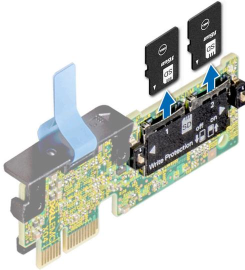
**Figure 96. Removing the MicroSD card**
