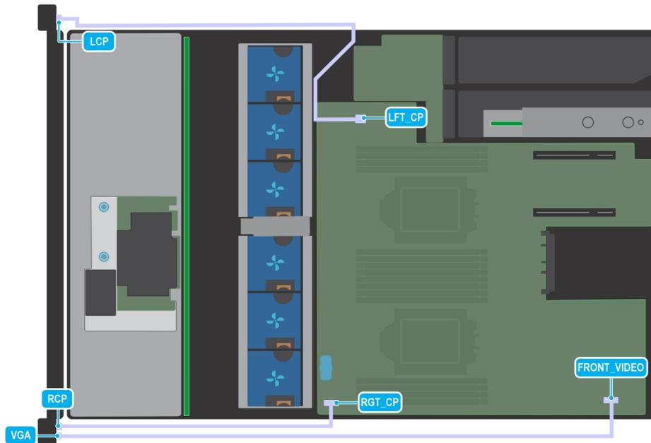
Figure 51. VGA and Control Panel
