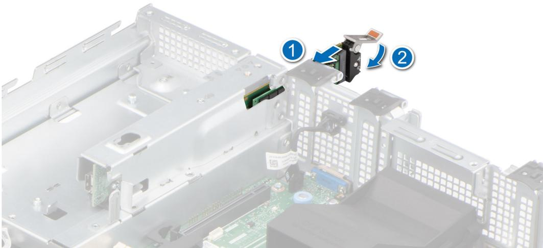
**Figure 85. Installing the BOSS S2 card carrier**
