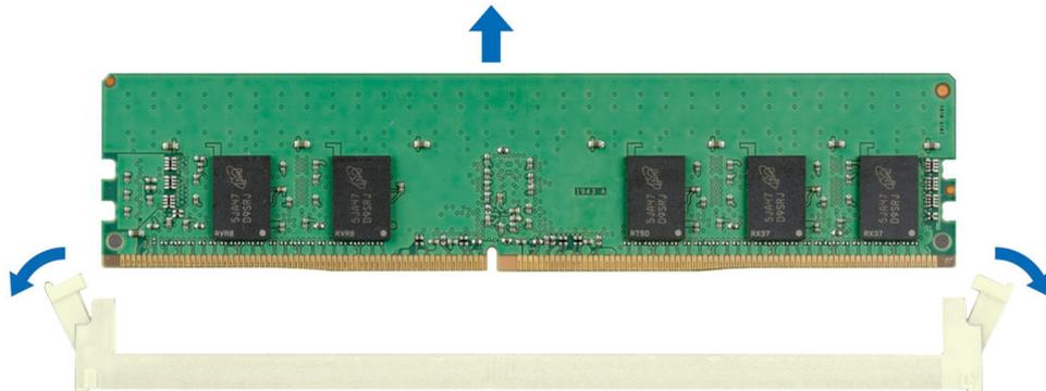
Figure 53. Removing a memory module
