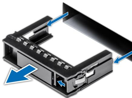
Figure 36. Removing a drive blank
