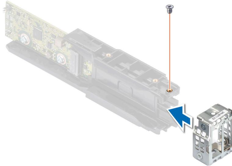
**Figure 80. Installing the BOSS cover**
