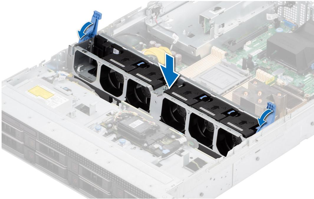
**Figure 27. Installing the cooling fan cage assembly**
