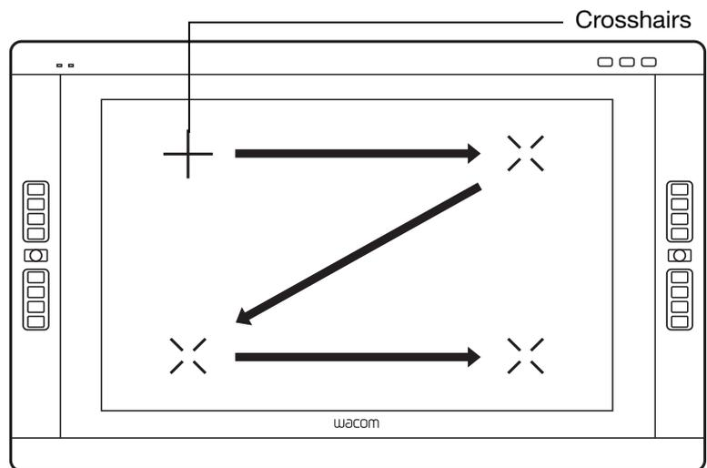
**Tip:** To see the screen cursor slightly offset from the actual position of the pen tip, calibrate by clicking on a spot showing that offset from the crosshairs. For example, to have the screen cursor appear 2.5 mm (1/10th of an inch) above and to the left of the pen tip, calibrate by clicking on a spot 2.5 mm (1/10th of an inch) below and to the right of the crosshairs.
