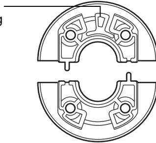
When correctly placed, the bearing stopper will shift smoothly from side to side within the stopper groove. The stopper will also sit flush with the rear hub surface.
