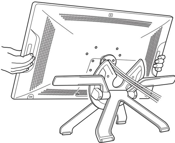
**Important:** When removing Cintiq from the display stand, always lift Cintiq in a direction parallel to the front of the stand. You may also need to slightly rotate Cintiq so the stand will release.
