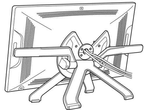
After mounting the pen display on the stand, remove the foam blocks that lock the adjustment levers in place. Save these blocks with the other packaging materials. You will need them if in the future you want to ship Cintiq.
