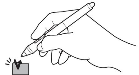
Press the upper side switch (when set to DOUBLE CLICK), or quickly tap the display screen twice in the same place with the pen tip. Double-clicking is easier when using the pen perpendicular to the pen display screen.
