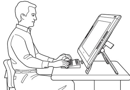
Adjust the stand to a more vertical position when a large amount of keyboard input is required. This position is also useful when presenting your work to co-workers or clients.
