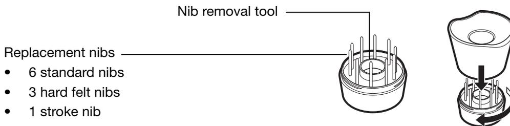
2. Clasp the old nib and pull it straight out of the pen. Use the nib removal tool, pair of tweezers, needle-nosed pliers, or similar instrument.
