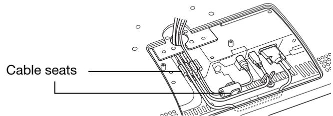
6. If the cable you wish to remove has thumbscrews, loosen them. Disconnect and remove the cable.
