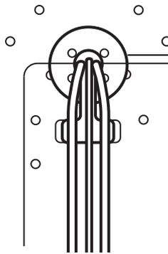
Proper positioning shows the hub sections aligned along the horizontal axis of the pen display.
