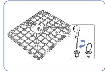
Tightly fasten the connecting screw at the bottom of the stand base.
