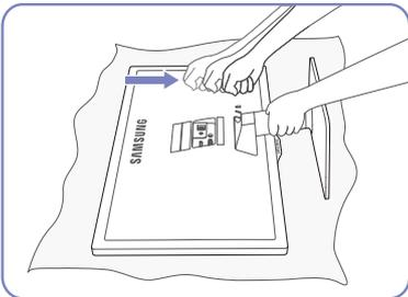
While holding the stand neck with one hand, pound the other fistful hand down onto the top of the stand base in the direction of the arrow to detach the stand base.
