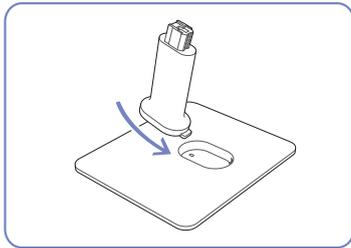
Insert the stand neck into the stand base in the direction shown in the figure.
