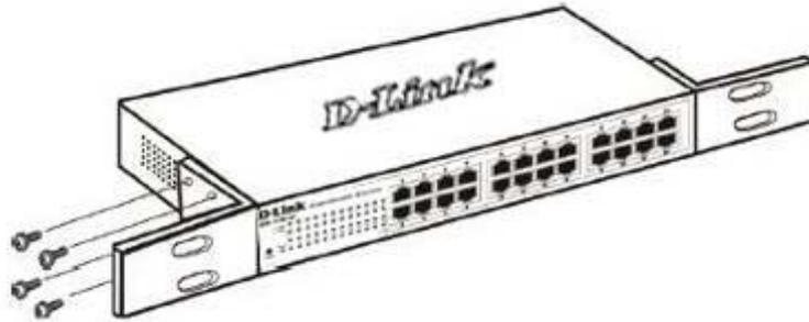
**Figure 8 – Attach the mounting brackets to the Switch**
