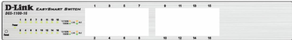
Figure 3 - DGS-1100-16 Front Panel
