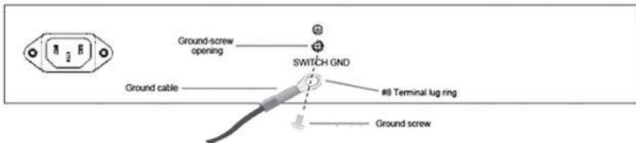
Figure 12 –Ground cable, screw and #8 terminal lug ring
