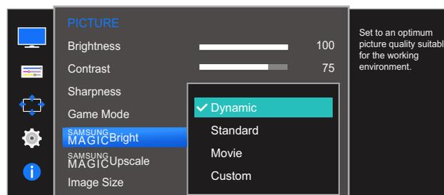
When the external input is connected through HDMI and **PC/AV Mode** is set to **AV**, **SAMSUNG MAGIC Bright** has four automatic picture settings (**Dynamic**, **Standard**, **Movie** and **Custom**) that are preset at the
