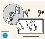
If the product generates a strange noise, a burning smell, or smoke, remove the power cord immediately and contact Samsung Customer Service Center (page 81).
